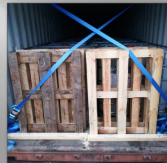
7. Cargo lashing inside container
