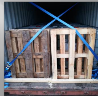
7. Cargo lashing inside container
